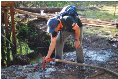
Soil Injection Method to combat against Peatland Fire
